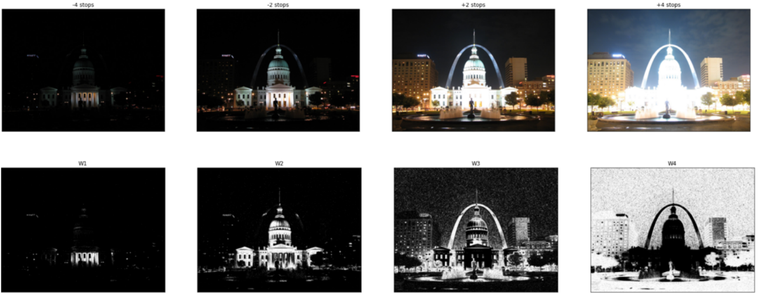
Figure 1: The input sequence (Top) and the corresponding weight maps (bottom) computed using equation (1). Image credits : Wikipedia
