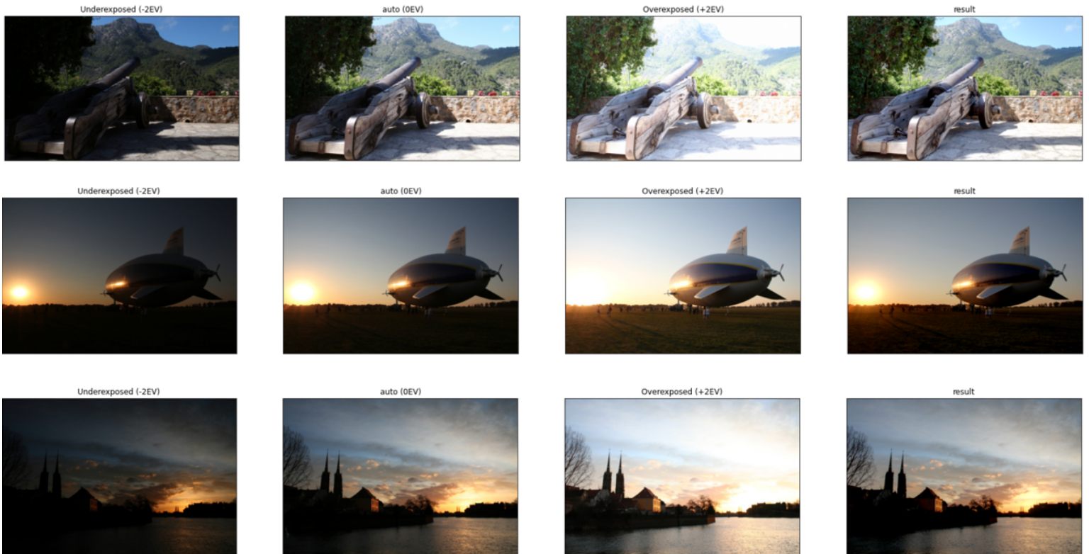
Figure 8: The input sequence (three first images) and the result of the multi-resolution exposure fusion (left).
